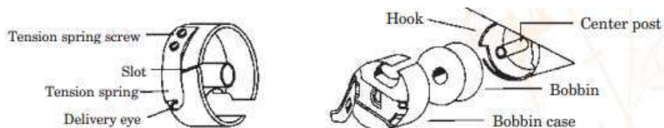
Fig:- 1.3.28. Bobbin case and bobbin mechanism
